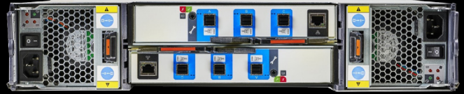
Figure 10: Seagate Exos E 2U12 Rear
