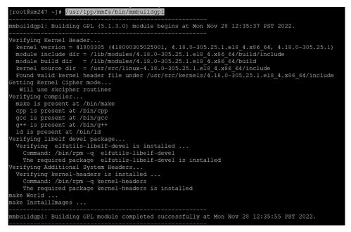
The example above shows that a Storage Scale portable layer was successfully created.
