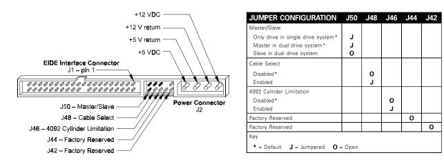
Figure 2-1 PCBA Jumper Location and Configuration
