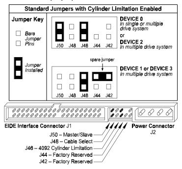
3 If the BIOS was set to AUTO DETECT, re-boot the system and use Max•Blast installation software to complete the hard drive installation. If other BIOS settings were used, access the system BIOS SETUP program and set the BIOS parameters to **Type 9** for the Maxtor hard drive then re-boot the system and use Max•Blast installation software to complete the hard drive installation. NOTE: When this jumper is installed, the Maxtor hard drive must be prepared using Max•Blast.
