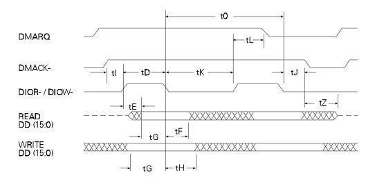
Figure 5 - 3 Multi-word DMA Data Transfer
