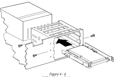
Figure 4 - 6 5.25-inch Installation
