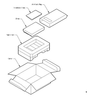
Figure 4 - 2 Single Pack Shipping Container (Option A)
