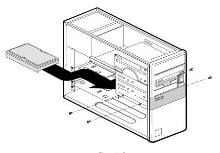
Figure 4 - 7 3.5-inch Installation
