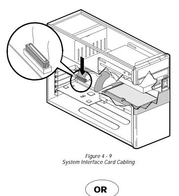
Attach the 40-pin IDE interface cable from the Maxtor hard drive to the IDE connector on the mother board.
