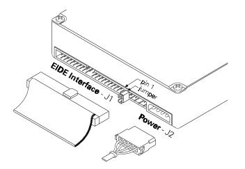
*Figure 4 - 8 IDE Interface and Power Cabling Detail*
