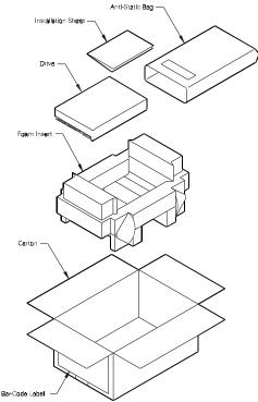
Figure 4 - 3 Single Pack Shipping Container (Option B)
