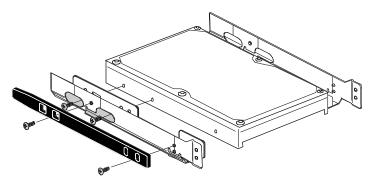
Figure 4 - 5 5.25-inch Mounting Brackets/Slider Rails
