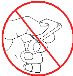
Figure 3. ST1.3 Series improper handling example
