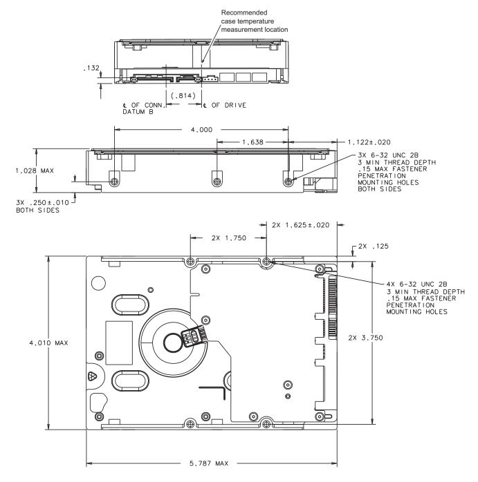
Figure 2. Mounting dimensions (2000GB model)
