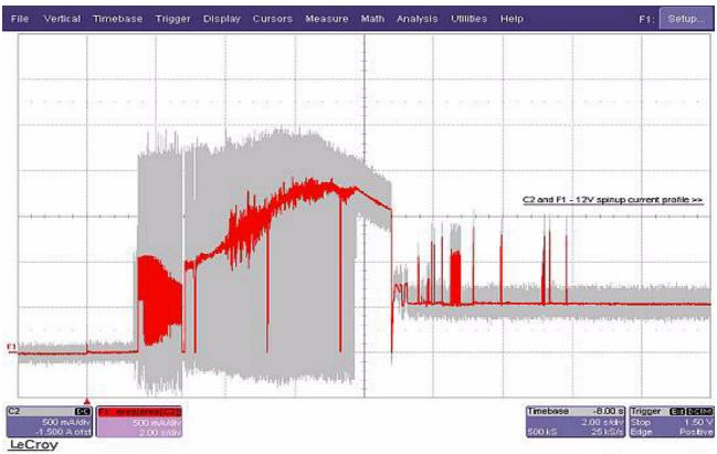
Note. Typical 12V startup and operation current profile
