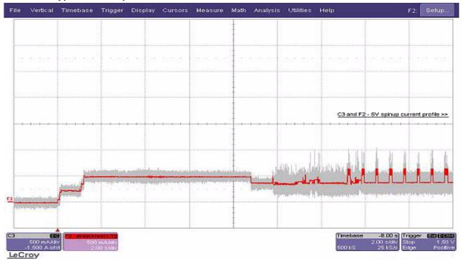
Note. Typical 5V startup and operation current profile
