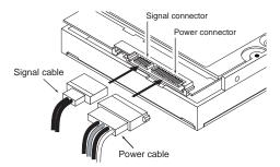
Figure 1. Attaching SATA cabling
