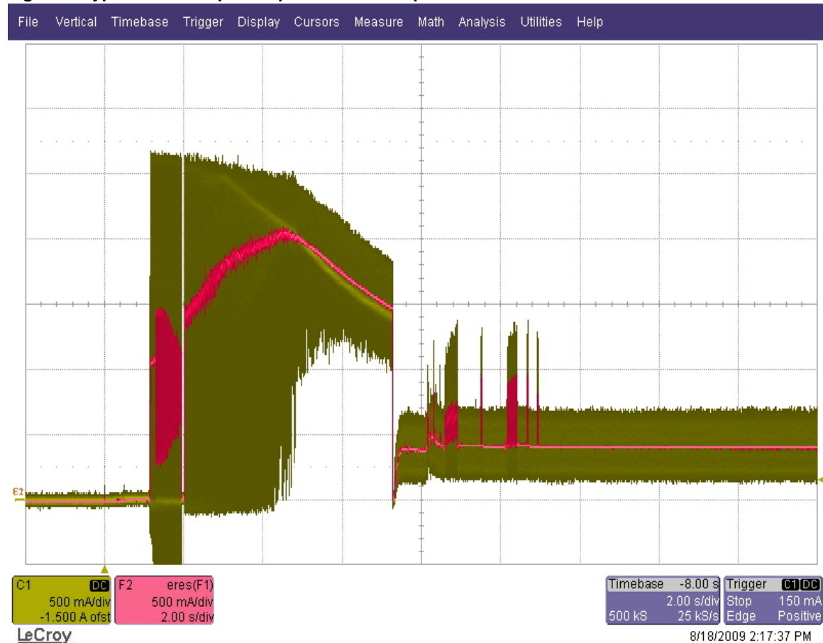
Figure 1. Typical 5V startup and operation current profile
