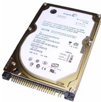
Figure 1. Momentus 4200.2 PATA disc drive
