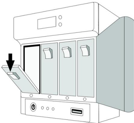
3. Press down on the orange button to release the failed drive from the server. If the server is powered on, wait until the drive stops spinning (approximately one minute) before continuing.
