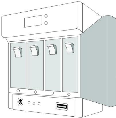
2. Locate the failed hard drive. Ensure that there is no activity on the drive by checking its LED—it should not be illuminated.
