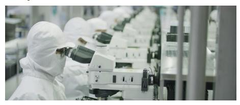
The testing process is long, complex, and manually intensive. There are 100,000 sliders in every 200mm wafer that need to be checked. The Normandale factory takes millions of microscope pictures every day, generating 10TB of data that must be sifted to detect potential production defects before wafers are assembled into drives.
