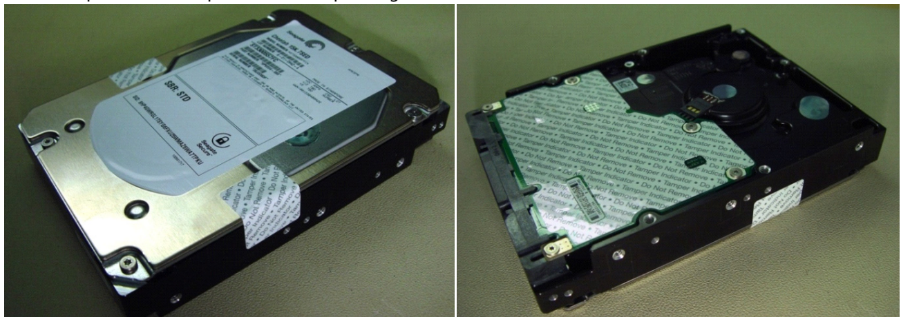
Figure 8. Example of FIPS tamper evidence labels.
