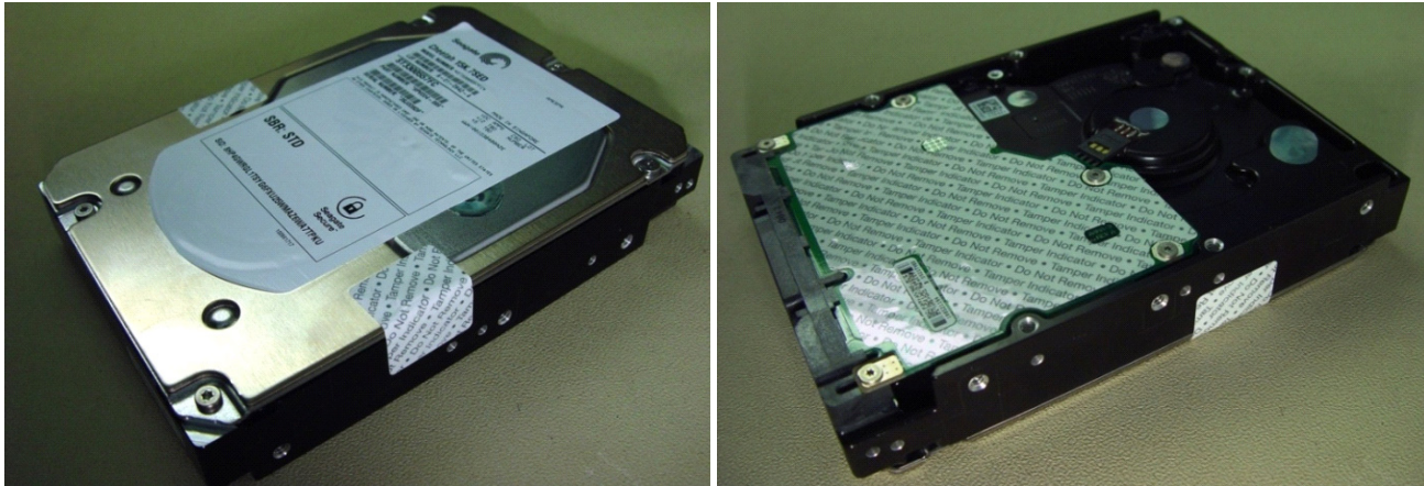
Figure 14. Example of FIPS tamper evidence labels.
