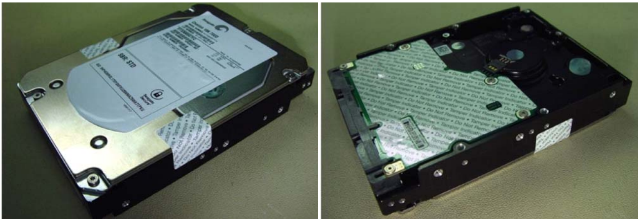
Figure 12. Example of FIPS tamper evidence labels/seals.
