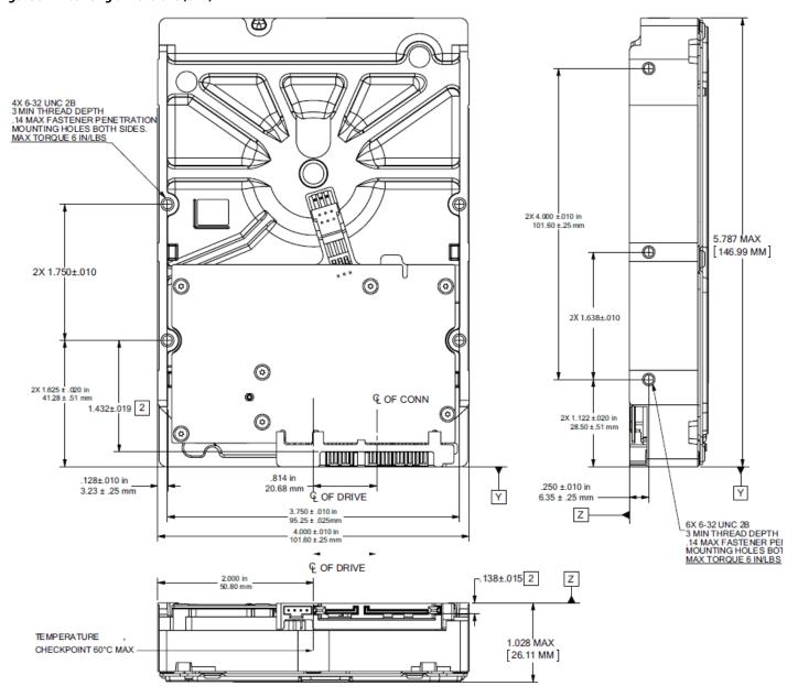
Figure 6 Mounting dimensions (4TB)
