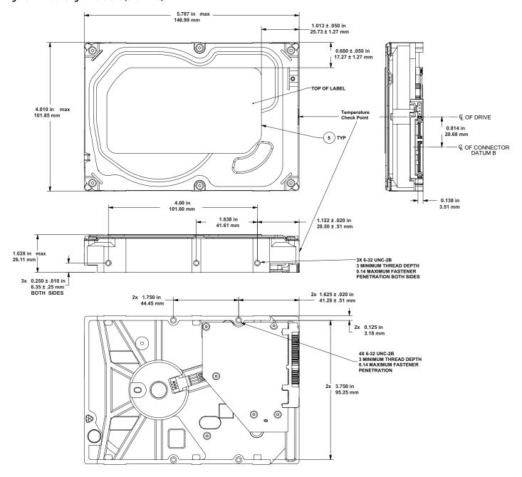
Figure 8 Mounting dimensions (1TB)
