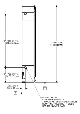
Figure 5 Mounting dimensions (6TB)
