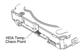
Figure 2 Location of the HDA temperature check point
