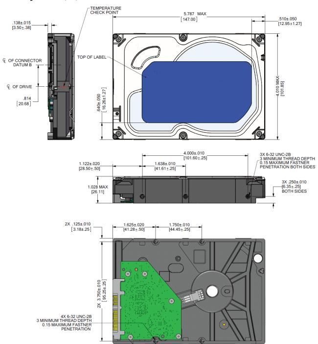
Figure 7 Mounting dimensions (3TB - 2TB)
