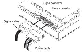
Each cable is keyed to ensure correct orientation. IronWolf drives support latching SATA connectors.
