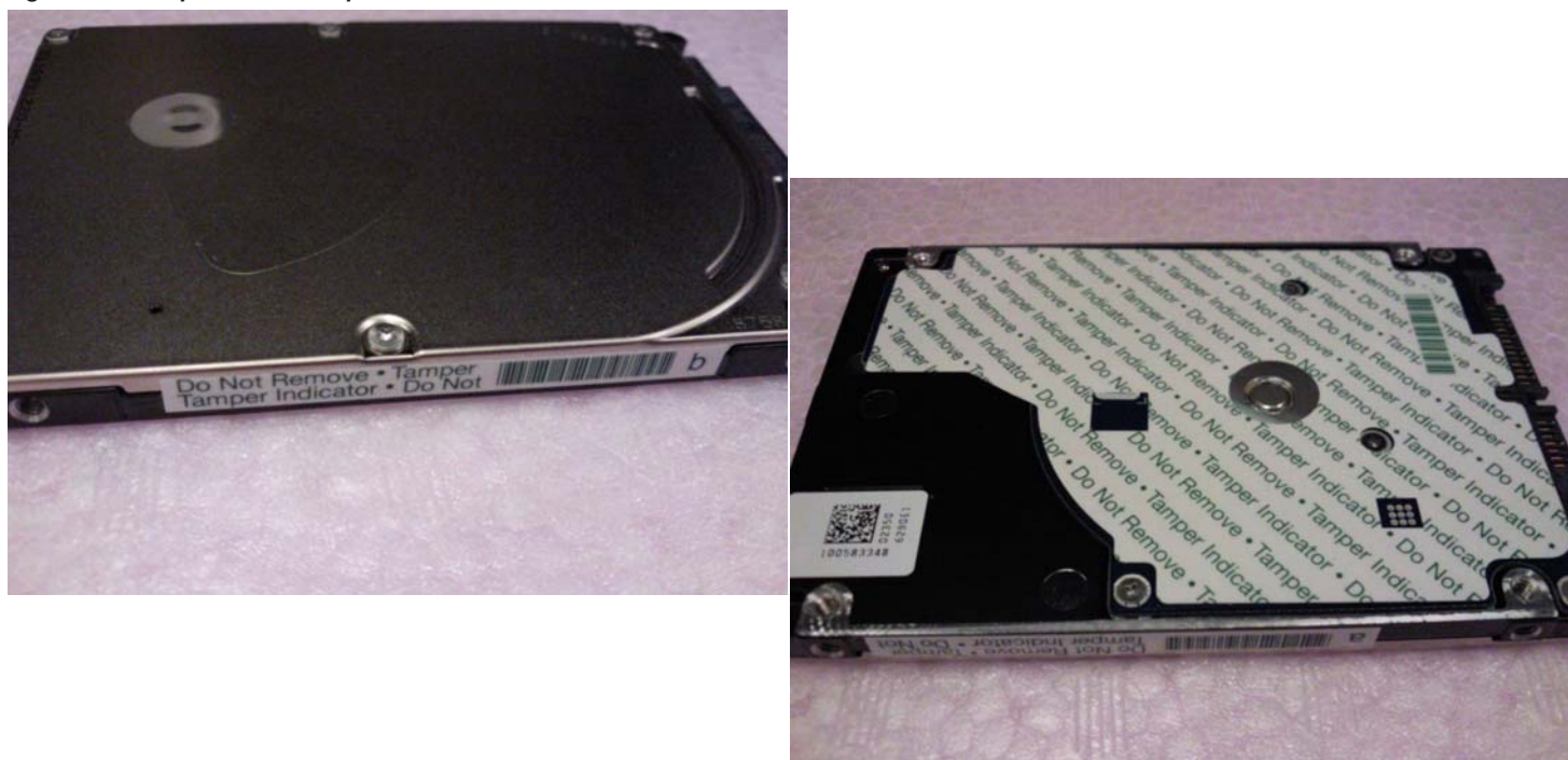
Figure 5 Example of FIPS tamper evidence labels.
