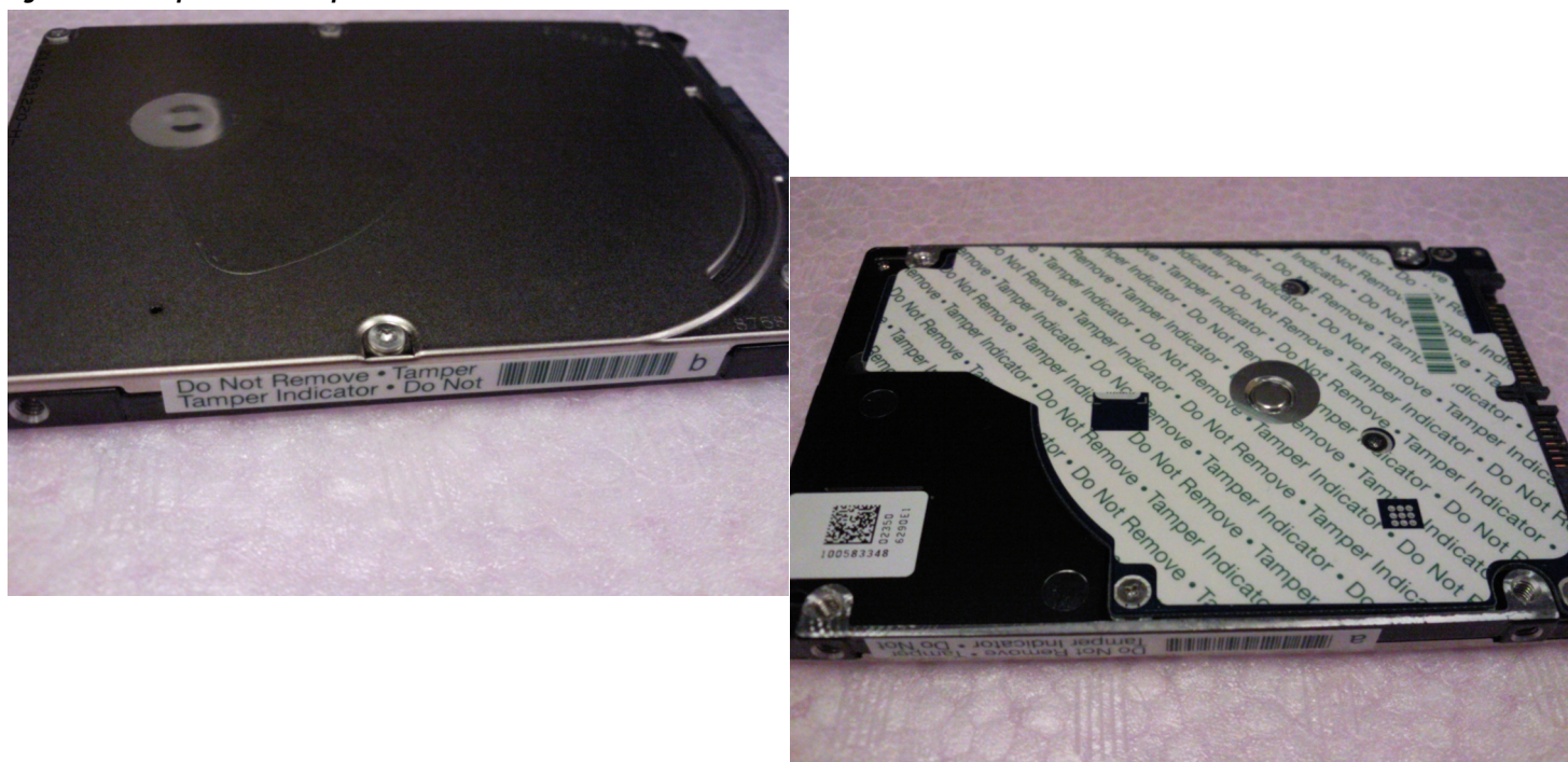
Figure 7 Example of FIPS tamper evidence labels.
