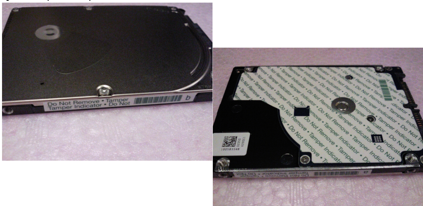
Figure 7 Example of FIPS tamper evidence labels.
