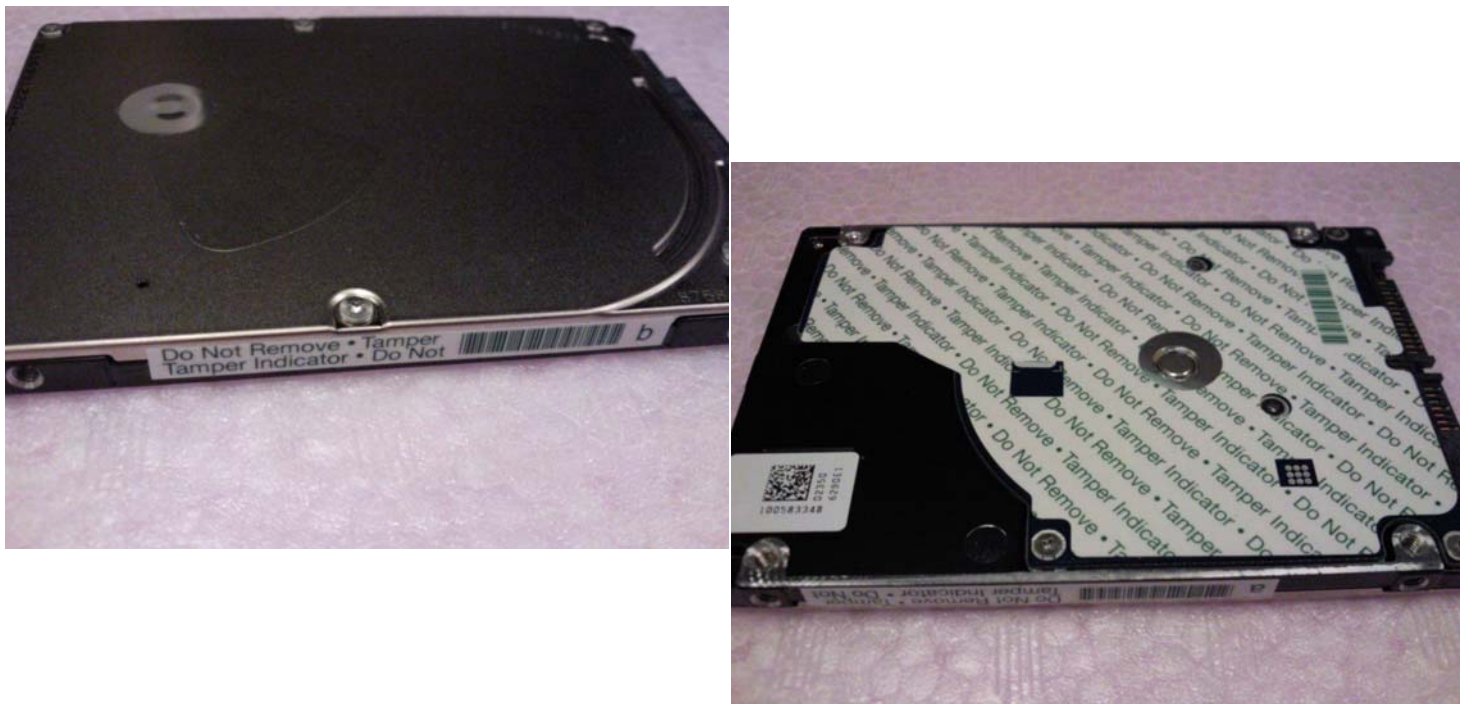
Figure 5 Example of FIPS tamper evidence labels.
