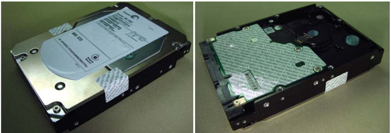
Figure 26. Example of FIPS tamper evidence labels.
